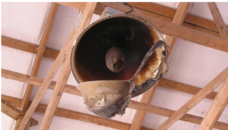
Figure 2.2. Light fixture in a dairy barn that caught fire due to the presence of a bird's nest (proximity of combustibles).
